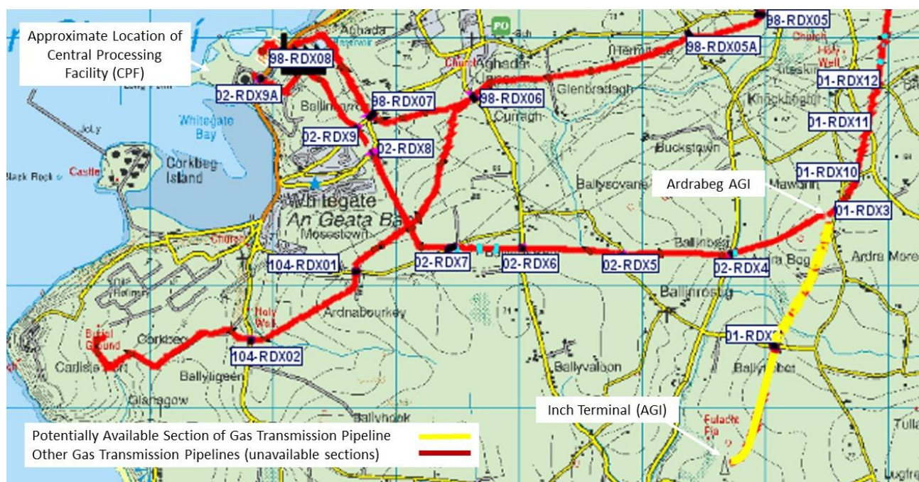
Figure 2-2 Section of existing Gas Pipeline that was considered for repurposing for CO 2 transmission
